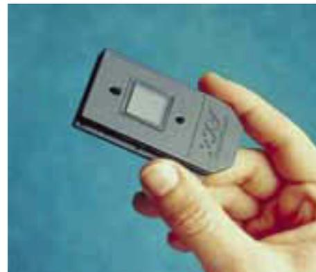
Figure 17.16 Affymetrix GeneChip® probe array (courtesy of Affymetrix)
