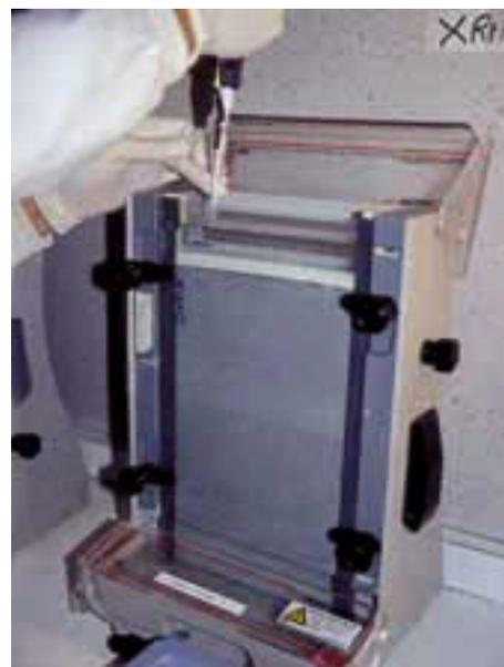
**Figure 17.11** Loading PCR-amplified DNA onto an SSCP/heteroduplex gel
