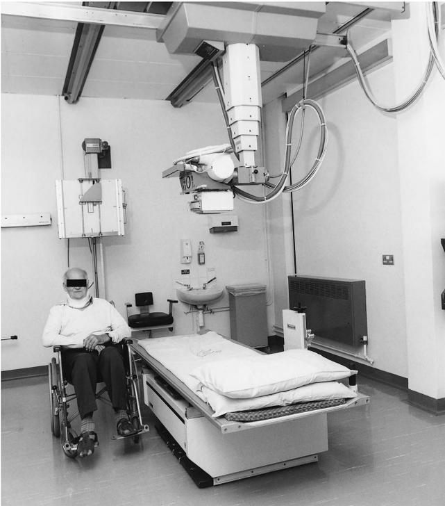
**Figure 2** Elevating adjustable height, floating table top X-ray examination table
