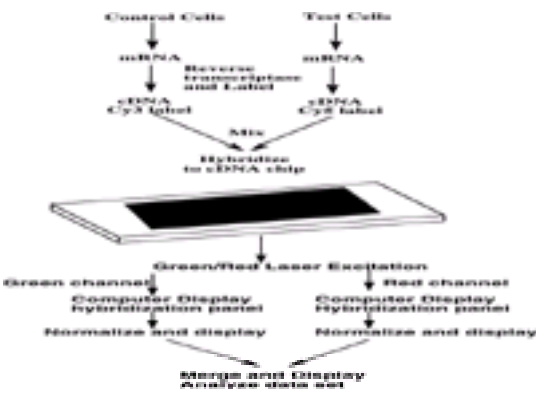
FIGURE 1.44. Diagram of a microchip array illustrating a typical experiment in which a set of control and test DNA are being compared to define transcriptional changes that result from a given test experiment. The cDNA is labeled, mixed, and hybridized to the oligonucleotides that have been precisely placed on the chip. Two different frequency lasers are used to excite the hybridized cDNA. Thereafter, emission from each x-y coordinate is collected, stored, and processed for further interrogation as to new or changes in transcribed genes.
