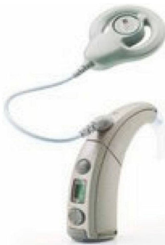
Figure 20.7 Nucleus cochlear implant (Cochlear Corporation) with ear level speech processor.
