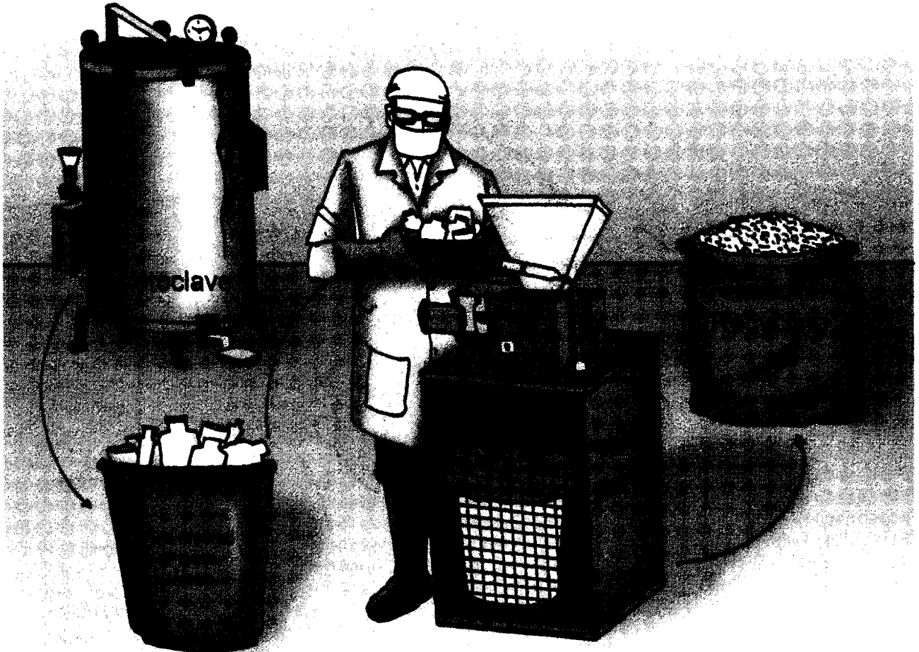
Disinfection and shredding of plastics
