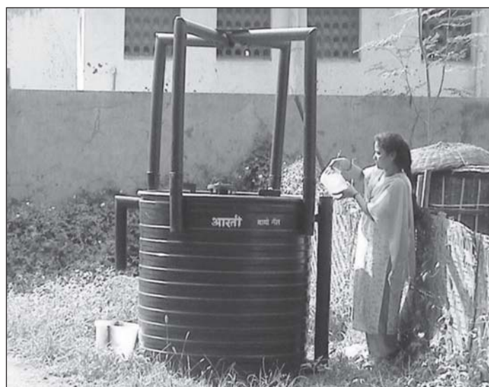
Fig - 18 : Portable Biogas Plant
