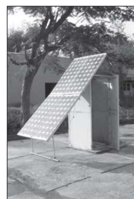
Fig - 15 : Temperature controlled Biodigester
