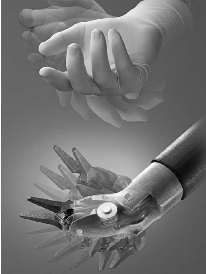
Figure 5–2. EndoWrist instrument allows for the reproduction of the human hand dexterity. (Courtesy of Intuitive Surgical Inc.)
